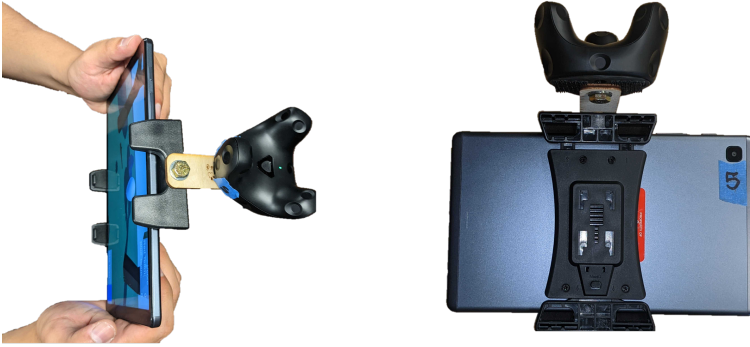
Fig. 2. Tracker mounted on a mobile device: top view (left) and back view (right)
