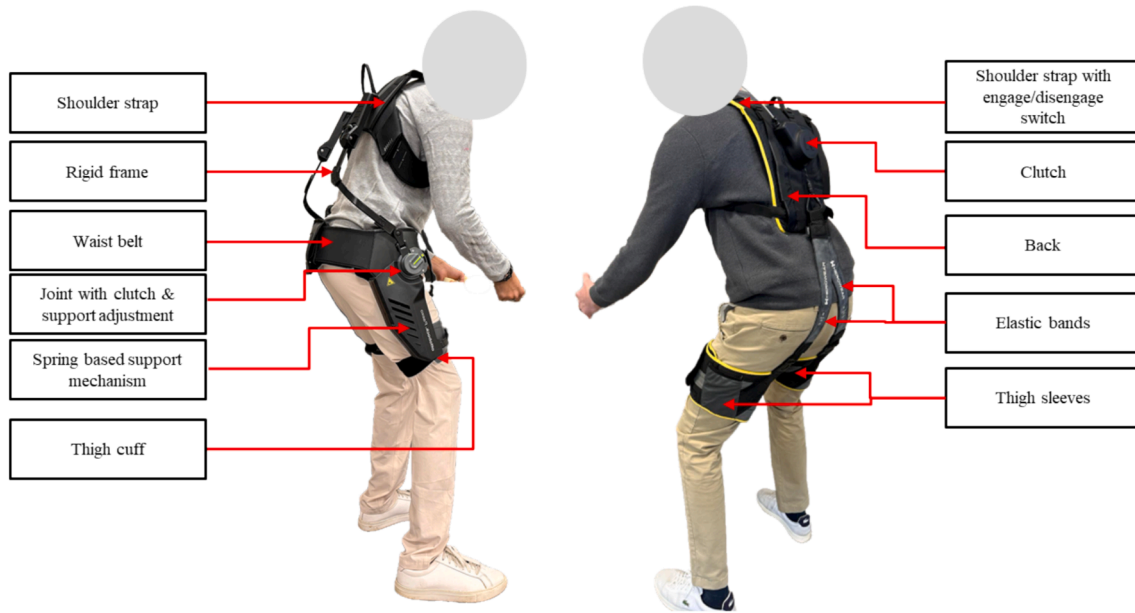
Fig. 1. Paexo Back (rigid) (left) and Herowear Apex (soft) (right) passive back-support exoskeletons.
