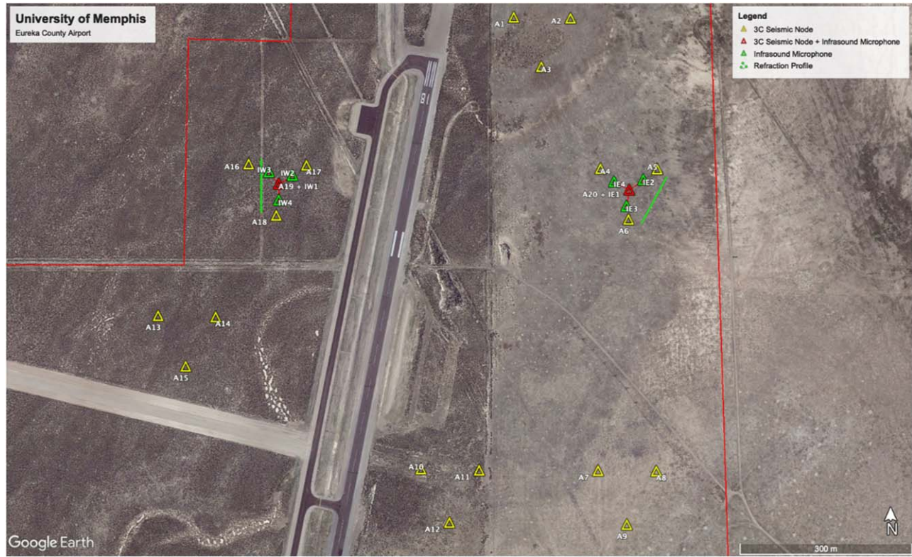
Figure A15. University of Memphis seismoacoustic array experiment. Yellow triangles show the location of the three-component seismic nodes in the Golay 3 \times 6 array configuration (A1–A18). Red triangles show the center infrasound instrument and colocated three-component seismic node for the western and eastern infrasound arrays (A19 + IW1, A20 + IE1). Green triangles show locations for infrasound microphones. Green lines show locations for the P and SH refraction profiles near the western and eastern infrasound arrays. The red lines show the boundary of the airport property.
