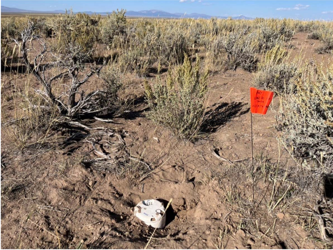
Figure A4. One of the seismic nodes deployed by JHU at the Beans Flat Rest Area (photo credit: B. Fernando).
