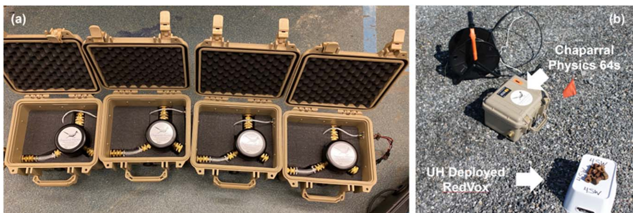
Figure A8. (a) Photo of the four Chaparral Physics 64s sensors in their cases before the OSIRIS-REx SRC reentry deployment. (b) One of the Chaparral Physics 64s sensors deployed near a RedVox sensor deployed by UH (photo credit: B. Elbing).
