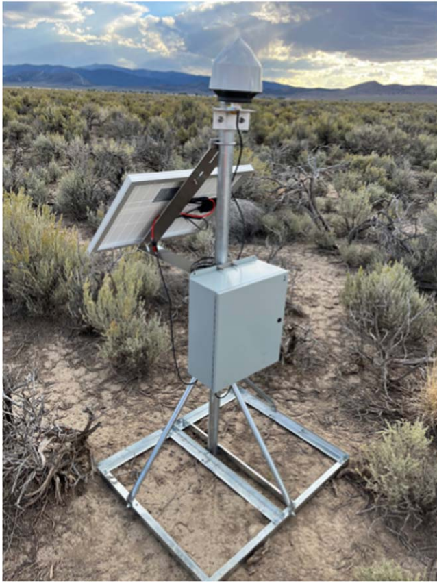
Figure A3. GPS ground station: Rex-2 (photo credit: R. Hasser).
