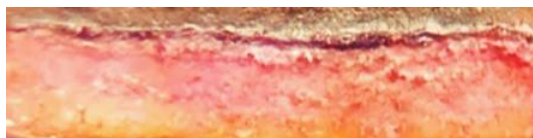
FIGURE 7 Dithizone stained ZnO on a fresh surface in the paint cross-section. The ZnO red stain correlated with the carbohydrate red-brown stain from TTC, suggesting a watercolor cake was used as a source of ZnO.
