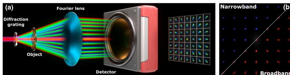
Fig. 1. BBSSP system and beam data comparison. (a) Broadband single-shot ptychography (BBSSP) system and false color beam image array. (b) Example of beam data, collected without the object in the system, for narrowband (top left) and broadband (bottom right) illumination.
