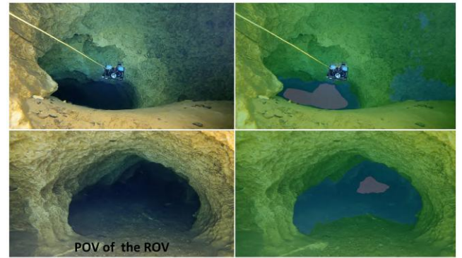
Fig. 6: A BlueROV2 is being teleoperated through a cave passage in Orange Grove, FL where the caveline is almost invisible; note that the yellow wire on the top image is the ROV's tether, not a caveline. In such scenarios, an AUV can leverage the segmented obstacles and open areas in the scene (overlayed on the right column) toward planning a trajectory to rediscover and follow the caveline.
