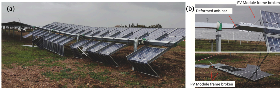
Fig. 11. Damage on a single-axis solar tracker due to wind-induced torsional load. Reproduced from Ref. Valentin et al. (2022) with permission from Elsevier, ©2022.
