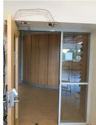
Fig. 3. 2.4 GHz and 5.8 GHz DR sensor mounted on top of a doorway [13].
