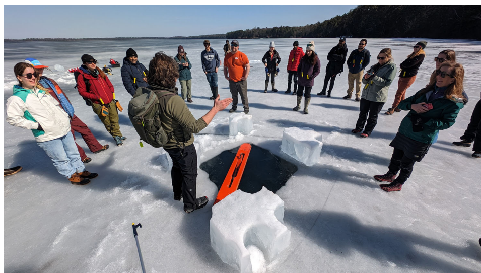
FIG. 2. Demonstrating the use of an ice jigger for running lines underice. Photo credit: Steven Sadro.
