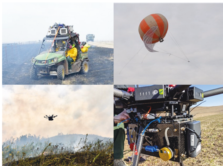
Fig. 1. Two Flyer sampling systems atop the ground-mobile XUV (top left), tethered aerostat carrying Flyer underneath (top right), and Kolibri sampling system attached to the undercarriage of the UAS (bottom left, in flight, and right, closeup).
