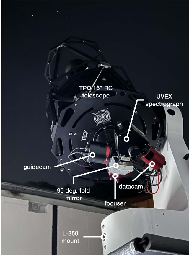
Figure 2. The assembled ArgusSpec optical train with key components labeled.
