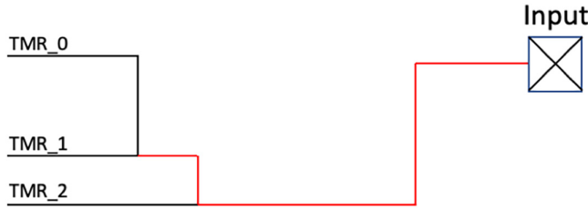
Fig. 5. Vulnerable segments of signal trunk originating from an untriplicated I/O.
