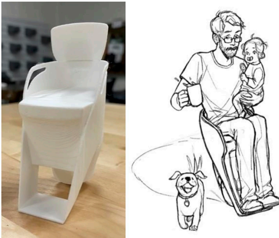
Figure 7. 3D-printed scale model of PURE (left) and illustration of PURE's hands-free driving capability (right).
