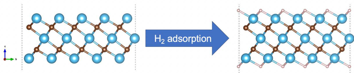
Figure 1. (a) Adsorption sites for hydrogen molecules as inspected from the top and side view. (b) The dissociation of H_2 molecule into the formation of Ti-H bond upon H_2 adsorption on a bare Ti_3C_2 surface.
