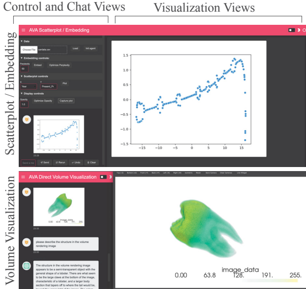
Figure 6: AVA integrated visualization interface. We implement AVA as a configurable system where individual components can be combined/configured for different target applications.
