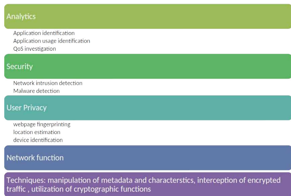
Figure 3. Encrypted traffic analysis and inspection phases.
