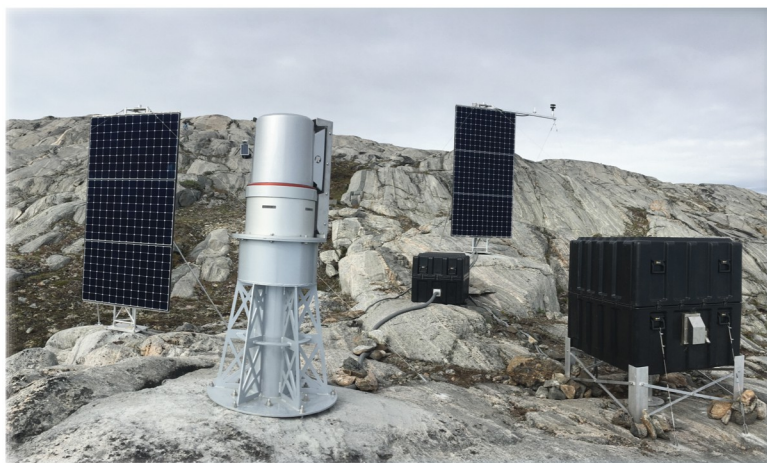
Fig 4. An autonomous terrestrial laser scanner system at Helheim Glacier, SE Greenland used to study calving dynamics (image credit: Cold Regions Research and Engineering Lab).
