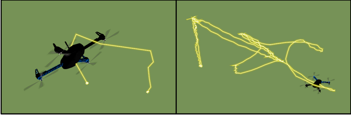
Figure 2: Left: crashing behavior caused by a configuration consisting of MC_PITCHRATE_P = 0.03, MC_ROLLRATE_P = 0.08 and MC_ROLL_P = 0.1. Right: a flight using the same configuration as on the left but with the addition of two parameter values: MC_PITCHRATE_K = 3.0 and MC_PITCHRATE_MAX=110.0.
