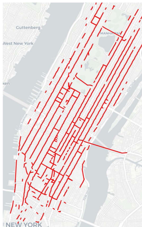
Fig. 3. Road segments for LSTM model training after two-step interpolation. (© OpenStreetMap contributors.)
