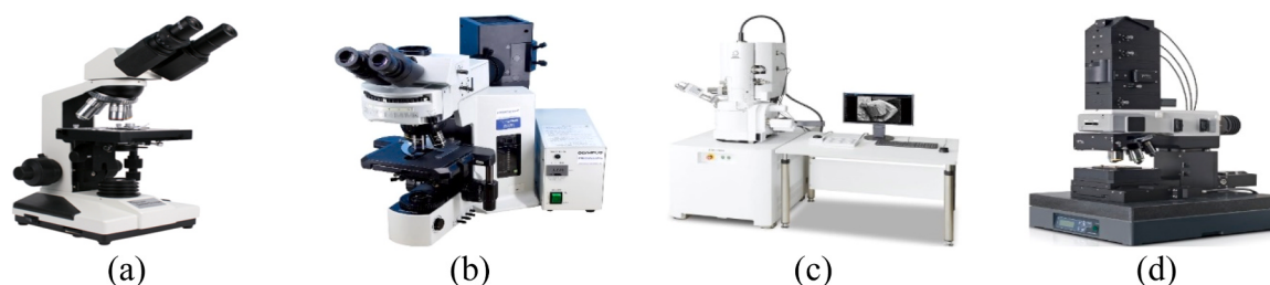
Fig. 8. Representative types of microscopes: (a) optical microscope, (b) fluorescence microscope, (c) scanning electron microscope, and (d) atomic force microscope.
