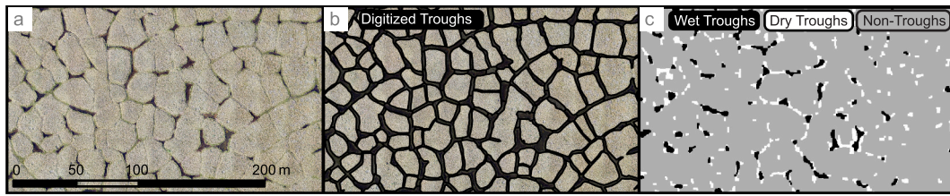
Fig. 7. Comparing drone-based and satellite-based methods of delineating ice-wedge troughs. (a) Drone orthomosaic image of South Site. (b) Hand-digitized trough boundaries in black on drone orthomosaic base map. (c) Satellite-derived trough map. Dry ice wedge troughs in white, flooded troughs in black, and non-trough area in gray.
