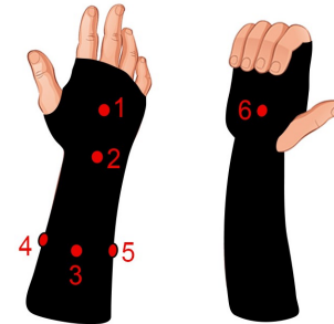
Fig. 4: Guidance sleeve with numbered vibrotactile motors
