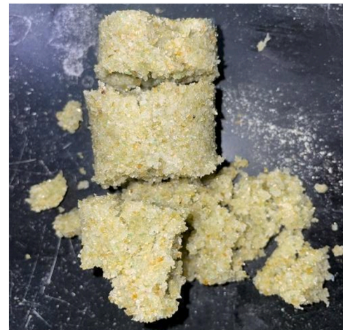
Fig. 7. The failure Alginate-treated sample with 20% mixing moisture content.
