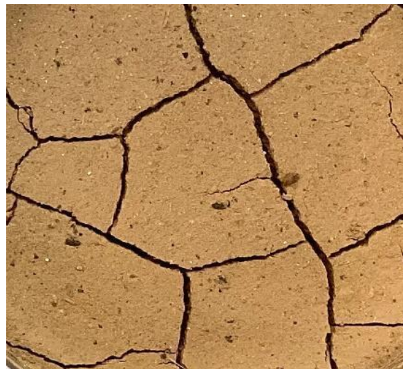
Figure 4. Typically untreated soil desiccation crack pattern.
