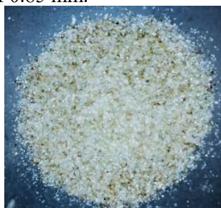
Figure 1. Recycled glass sand with a particle size of 0.85 mm.
