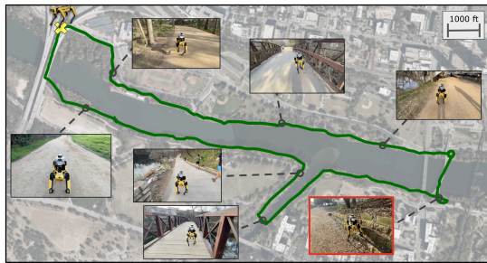
Fig. 4. Trajectory trace of a large-scale qualitative deployment of \text{PATTERN}^+ along the 3-mile trail. With only five minutes of supplementary data, \text{PATTERN} required only one manual intervention to stay on the trail and successfully completes the hike, demonstrating robustness and adaptability to real-world off-road conditions.
