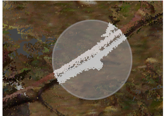
Figure 6: The highlight effect previewing the points that will be selected by a potential paint operation in the 2D interface. In this image, the depth limit feature is preventing the background points from being selected. The VR condition also has this highlight effect for points within the hand spheres.
