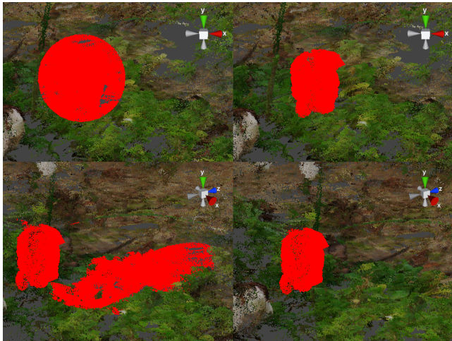
Figure 5: An example of the depth limiting algorithm used in the 2D system. The top images show the initial painted view. The bottom two images show the same cotton boll from a rotated perspective after the paint operation. The left two images have the depth limit turned off, and the right two have the feature turned on.
