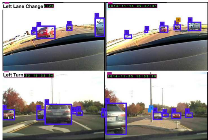
Fig. 3. Object detection pre-processing results on the Brains4Cars dataset [9]. The object classes Car, Bicycle, Person, Traffic Sign, and Traffic Light are mapped to classes 0, 1, 2, 3, and 4 in the images shown. Only these object classes are used.
