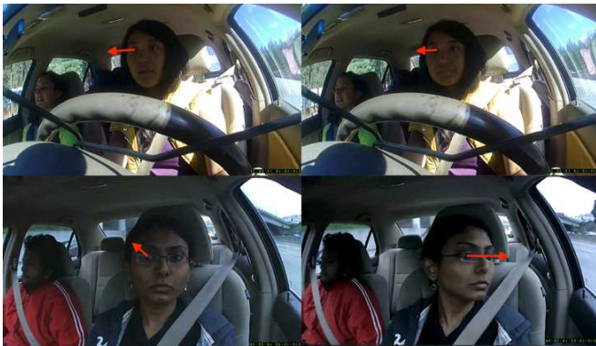
Fig. 2. Qualitative results of the gaze preprocessing algorithm on the Brains4Cars dataset. The red arrow projects their gaze to a point on the imaginary plane.
