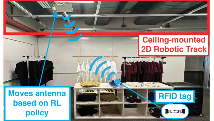
Fig. 1: RL2 - SAR-based robotic RFID localization system using RL. RL2 moves a ceiling-mounted antenna autonomously on a 2D track system. The antenna can move in x, y, and diagonal directions to perform Synthetic Aperture Radar (SAR) and localize RFID tags in the environment. It uses Reinforcement Learning to learn a strategy to localize multiple RFID tags in the environment more efficiently.
