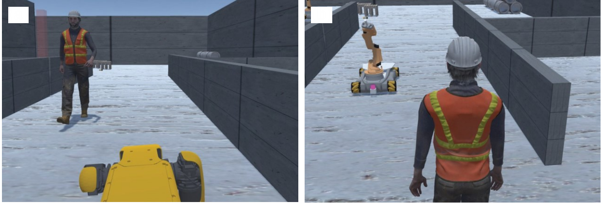
Fig. 4. Virtual construction site environment in Unity. Fig. 4(a) illustrates a trial when participants take a teleoperator role and navigate from a robot's point of view while encountering human NPCs. Fig. 4(b) illustrates a trial when participants take a human worker role and navigate from a human avatar's point of view while encountering robot NPCs.
