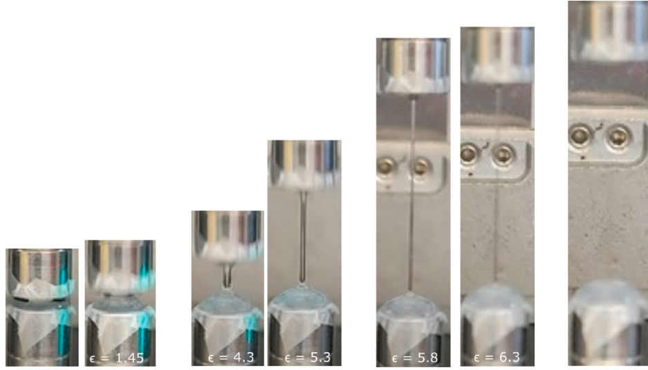
Fig. 1. Capillary necking and filament stretching of a dilute polymer solution on the VADER.
