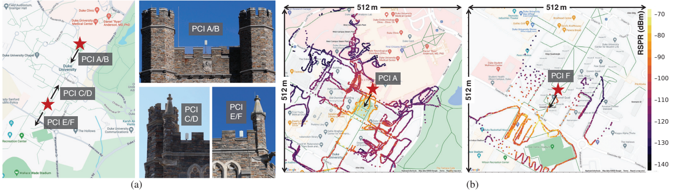
Fig. 4: (a) Six LTE cells operating in the CBRS band deployed on the Duke University West Campus (detailed cell information in Table II). (b) Sample RSRP measurements collected by the UE when served by two cells (PCIs A and F) within the 512 m x 512 m area.
