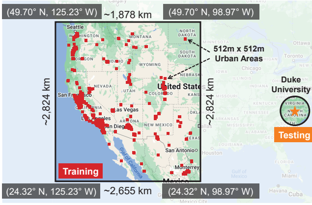
Fig. 3: A 6.41 million km 2 area in North America (left), from which a total number of 27,176 512m×512m areas with a building-to-land ratio of at least 20% are selected to generate the building map and PG map datasets used to train the cascaded U-Net model in GEO2SIGMAP. The trained model is evaluated using measurements conducted on the Duke University campus (right).
