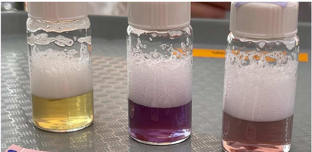
Figure 3. Vials with liquid solutions obtained from soil samples in process of lead screening. Source: the authors.
