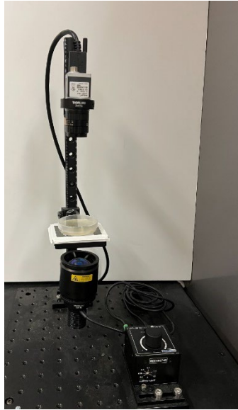
Figure 2. Automated behavioral analysis of C. elegans using Tierpsy Tracker. The Basler acA4024-29um camera captures high-resolution video of the nematodes, allowing Tierpsy Tracker to accurately track their movements and quantify various behaviors and locomotion patterns.
