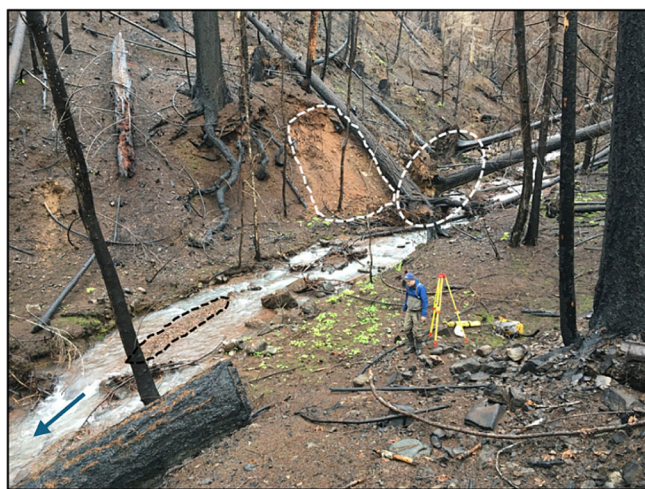
FIGURE 8 BOG study reach in December 2020, showing post-fire geomorphic change (inferred from observational evidence) including treefall, slumping, and a mid-channel gravel bar; blue arrow indicates flow direction. BOG, Bogus Creek.
