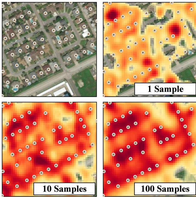
Fig. 6. Aggregated debris distribution (debris height) for various number of samples.
