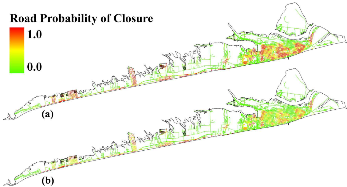
Fig. 8. Probability of road links closure in the aftermath of hurricane event considering both roadway infrastructure and debris impact for (a) normal vehicles; and (b) emergency vehicles.
