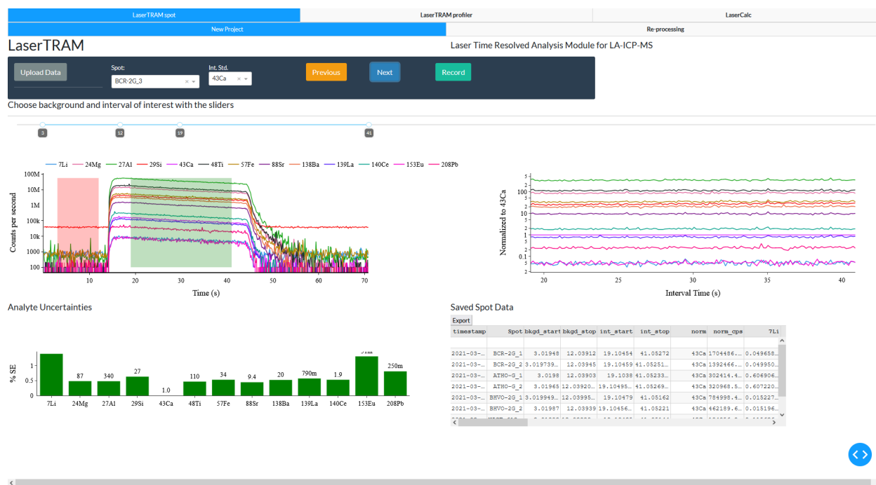
Figure 3: Example of the LaserTRAM New Project tab after data has been loaded in.
