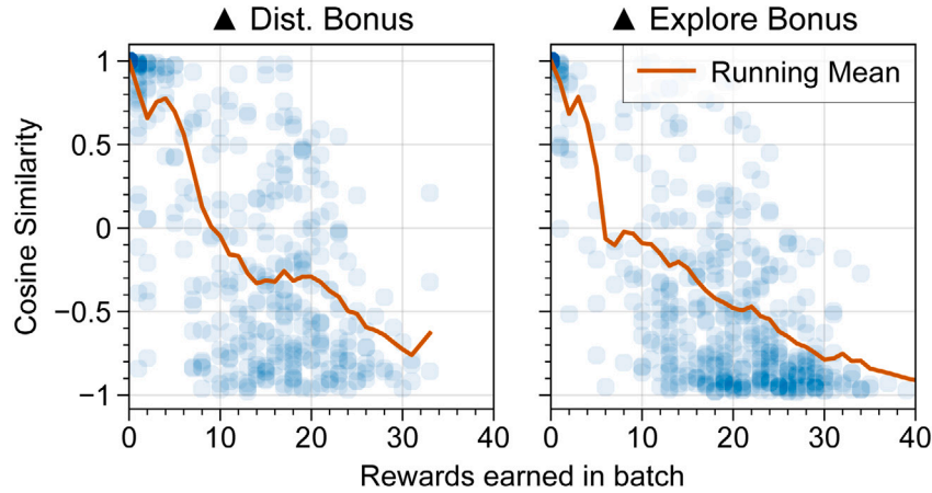
Fig. 12. Cosine similarities between RL gradients and pure reward gradients, organized by the number of goal rewards earned in the batch. Blue dots indicate the cosine similarities for individual batches. The orange line shows a running exponential mean of the cosine similarity measure. Only agents trained with 1600 batch size are shown.
