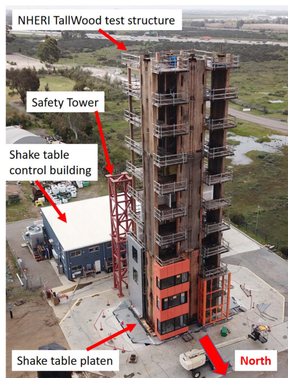
Fig. 1. Full-scale 10-story NHERI TallWood test structure with rocking wall lateral system. (Image by authors.)
