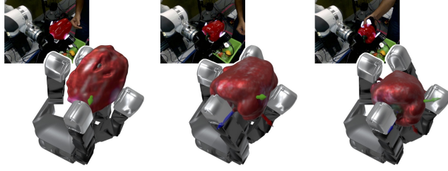
Figure S18: Visualization of pose drift. We illustrate the pose drift in two separate bell pepper experiments, with final pose metrics of 5.8mm and 8.24mm respectively. In the second experiment, the object is upside down with poor visibility, and this is reflected in the growing pose drift.
