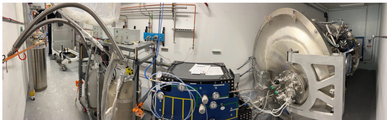
Figure 5 KPF instrument along with the vacuum cart and cryogenic fill system. A 180L shown temporarily secured to the wall that feeds two 50L dewars on a cart. Two pumps circulate LN2 from the 50L dewars to the cold heads on the blue and red detectors.
