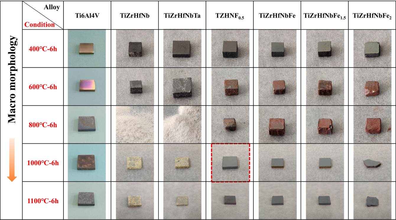
Fig. 1. The macroscopic-surface characteristics of RHEAs with different compositions as well as the Ti6Al4V alloy after oxidation at temperatures ranging from 400 °C to 1100 °C for 6 h.
