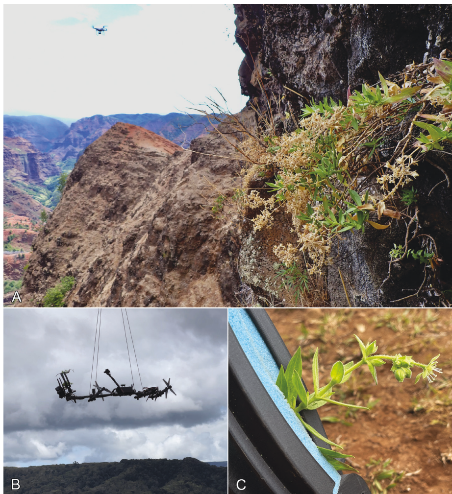
Figure 4. Collecting Schiedea waiahuluensis via drone A population accessed on rope, with drone in background William AMW821, photo by Adam Williams B collecting arm hanging from drone, photo by Ben Nyberg C drone collecting arm with specimen, Nyberg BN023 photo by Ben Nyberg.
