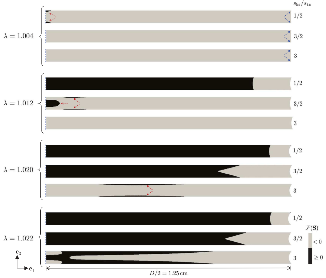
Fig. 3. Contour plots, over the deformed configuration, of the regions of the specimen where the stress field exceeds ( F(S) \geq 0 ) the Drucker–Prager-type strength surface of the elastomer at four increasing values of the normalized global deformation \lambda = h/H between the fixtures. The results correspond to specimens with a diameter-to-thickness ratio D/H = 40 and an elastomer with uniaxial tensile strength s_{ts} = 0.24 MPa and the three different values of hydrostatic strength s_{hs} listed in Table 1, so that s_{hs}/s_{ts} = 1/2, 3/2, 3 . The plots are shown only over half of the specimen for better visualization.
