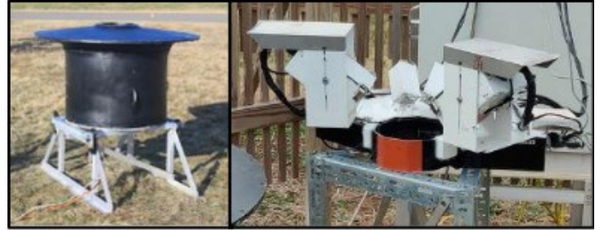
Figure 1. Snowflake Measurement and Analysis System (left) and Multi-Angle Snowflake Camera (right).
