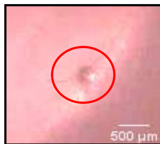
(d) Selected sequences of images in Test C illustrating the third interior crack nucleation, and three-crack interaction.
