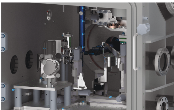
Figure 8. The chemRIXS instrument close-up view inside the sample chamber. This chamber was modified to house an electromagnet and cryostat sample holder to perform XPFS studies on solids.
