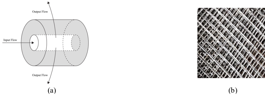
Figure 1: (a) Jelly roll configuration. (b) Stacked structure of Microlith.
