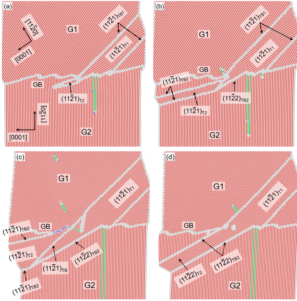
Fig. 3. (a) Nucleation of a second (11\bar{2}1) twin from the tip of the first one, but it grows into G2. The TB is denoted as (11\bar{2}1)_{TB2} . (b) As the (11\bar{2}1) twin in G2 grows, the tip of the first (11\bar{2}1) twin in G1, which is part of the GB, is evolving into a coherent (11\bar{2}2) TB (denoted as (11\bar{2}2)_{TB2} ), with respect to G2. (c) The coherent (11\bar{2}2)_{TB2} extends further down into G2, forming a special twin configuration: above the GB, the twin is a (11\bar{2}1) twin with respect to G1, whereas across the GB, the same twin is a (11\bar{2}2) twin with respect to G2. The first (11\bar{2}1) twin which is with respect to G1, and the second (11\bar{2}1) twin which is with respect to G2, also satisfy the (11\bar{2}1) twin relationship. (d) Eventually, the second (11\bar{2}1) twin disappears, and two coherent (11\bar{2}2) TBs (denoted as (11\bar{2}2)_{TB2} ) are formed, both with respect to G2.
