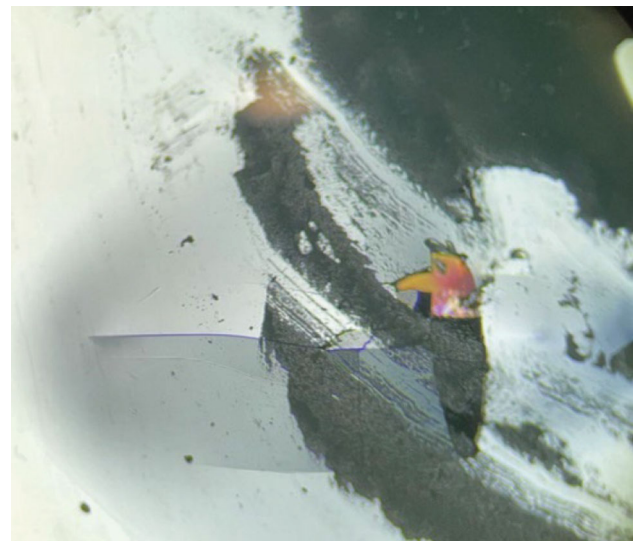
Fig. 11. Damage on the silicon back surface after thinning
