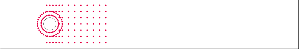
FIG. 7. Initial candidate sensor positions for the confined cylinder flow. The box represents the spatial domain used in the simulation.
